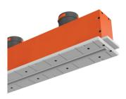
PROFILE 600 VERTICAL model diffuser is specifically designed for installation on the "face" of the plasterboard ceiling. It connects to a flexible 75 mm plastic duct system and requires only 17 cm of space for installation.
